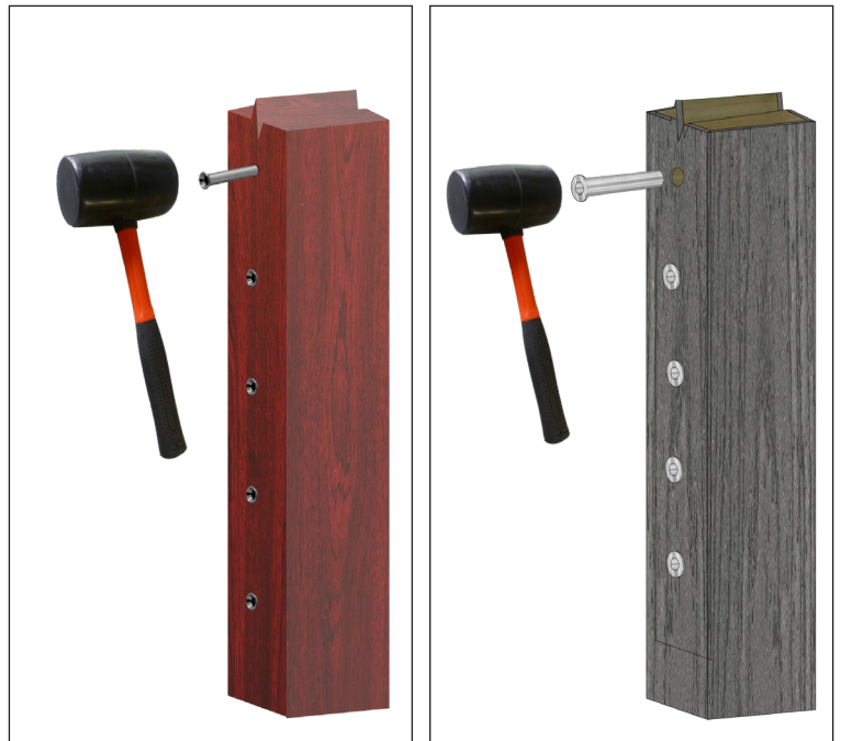
Figure C. Tap Cable Sleeves snugly into place (wood mid post on left and composite mid post on right).
