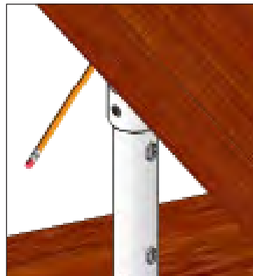
Figure AY. (LEFT) Mark screw holes in the cable stabilizer adjustable base with a pencil.
