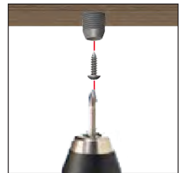
Figure H. Assemble the Aluminum Stabilizer Kit by attaching the base plate to the connector block.
