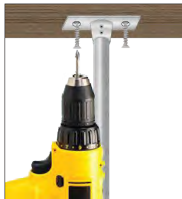
Figure Z. (LEFT) Attach the top of the stabilizer to the underside of the top rail with (2) two 1/4 x 2" flat head wood screws. Figure AA. (RIGHT) Attach the bottom of the stabilizer to the mounting surface with (2) two 1/4 x 2" flat head wood screws.
