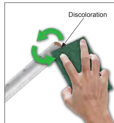
Figure AF. (LEFT) Remove any surface discoloration with a Scotch-Brite Pad.
