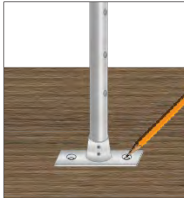
Figure AL. (LEFT) Mark screw holes in the lower stabilizer base with a pencil.
