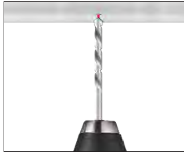
Figure AJ. (LEFT) Mark with a marker the center position.
