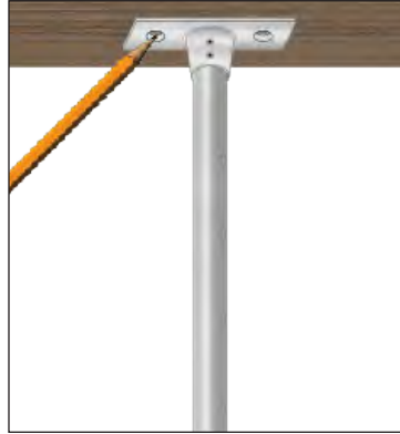
Figure V. (LEFT) Mark screw holes in the upper stabilizer base with a pencil. Figure W. (RIGHT) Mark screw holes in the lower stabilizer base with a pencil.
