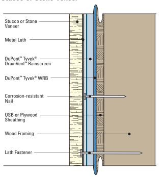
Prior to installation of stucco system or stone veneer, attach metal lath over DuPont™ Tyvek® DrainVent™ Rainscreen in accordance with manufacturer's recommendations and the requirements of ASTM C1063. Install casing beads and other accessories for stucco/ stone veneer at top of wall, cladding transitions, around windows/doors, etc. per specifications and manufacturer's instructions. Install stucco system or stone veneer according to the manufacturer's recommendations.
