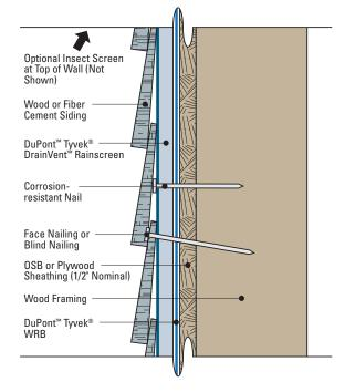
Install wood siding or fiber cement cladding over DuPont™ Tyvek® DrainVent™ Rainscreen in accordance with the cladding manufacturer's recommendations.
