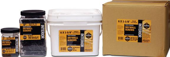
Screw Products, Inc. is proud to offer our new, high quality, drywall screw line featuring sizes from a #6 X 1-1/8" to a #8 X 3". Our drywall screws have a bugle head to prevent tearing, a phosphate coating to help resist corrosion and a Phillips drive recess. They are excellent for wall board, drywall, plaster board, sheet rock, gypsum board, and other materials. Our screws are packaged in 1lb jars, 5lb jars, Bulk Pails and 50lb boxes. They are great for any size project.
