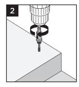
NOTE: Drive the screw in all at once, do not stop. You will hear a change in sound when the screw is fully driven.
