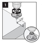
Using the HEXSTIX® depth setter in a 18v or greater drill or impact driver, install fasteners at a 90° angle (perpendicular to the board). Drive the screws into the decking until the bit releases from the screw.
