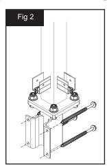
Using the appropriate lag screw bolts for your application (sold separately), attach the post and fascia bracket assembly to the structure as per local building codes (see Fig 2).
