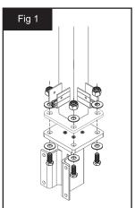
Secure the base plate of the post to the top plate of the fascia bracket using the supplied hardware (see Fig 1).
