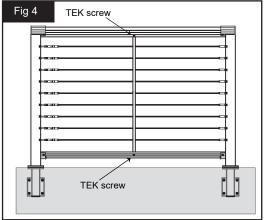
An alternative to using a fascia mount bottom rail support bracket on picket or cable railings is to place a TEK screw through the side of the top and the side of the bottom rails where the intermediate picket intersect (see Fig 4).
