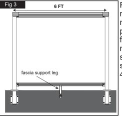
For our frame glass railings, the maximum space between posts is 6ft (72"). A fascia mount bottom rail support bracket should be used on spans greater than 48" (see Fig 3).
